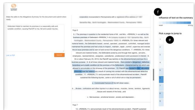
Figure 2. The UI built for testing, attention highlights condition. The highlights in the full case text viewer have many shades of blue. (e) An average attention score was computed per page and min-max scaling was applied to normalize the scores for the Jump-to-page functionality. As a result, the higher the score, the more intense the shade of the highlighting of the page in the index. (f) A scale was added to the UI to explain how to read the highlights.
