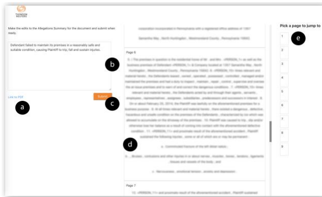
Figure 1. The user interface (UI) built for testing, no highlights condition. (a) Link to the full case source text in the original PDF format. (b) A text field area to view and edit the summary generated by the model. (c) Submit button which stopped the timer and made a pop up appear where the participant could leave comments before the next case was displayed. (d) Source text viewer displaying the OCR'd source document of the case. (e) Jump to page functionality - each rectangle represents a page of the source document
